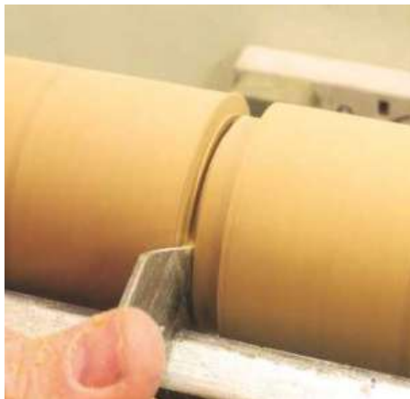
▲ Pic.5 After deciding where the lid is going to be cut in about 10mm deep and 10mm wide for the spigot, make an incision with the 1.5mm parting tool to mark the cutting-off point
